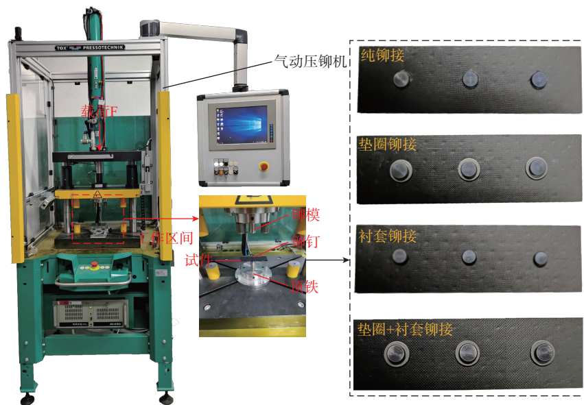
图4 铆接装置及铆接后试件 Fig.4 Riveting setups and specimens after riveting
